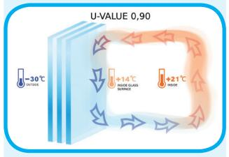
Convection is caused by the air temperature close to the window being lower than in the room. Cold air descends, moves across the floor and rises back up, causing a sensation of draft and cold radiation. When glass is heated just one or two degrees higher than room temperature, it stops convection and draft
