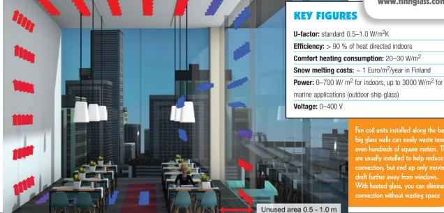
Fan coil units installed along the base of big glass walls can easily waste tens or even hundreds of square meters. They are usually installed to help reduce draft further away from windows. convection without wasting space
